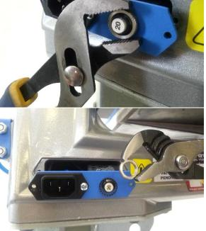
Remove old Circuit Breaker and discard by unscrewing silver mounting ring, using pliers if necessary
