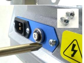
Install new Circuit Breaker by screwing on toothed washer and silver mounting ring, noting amperage rating orientation as shown
